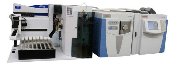
Tekmar Atomx XYZ Purge & Trap (P&T) coupled with the Thermo Scientific<sup>™</sup> ISQ<sup>™</sup> 7000 GC-MS System and Thermo Scientific<sup>™</sup> TRACE<sup>™</sup> 1310 Gas Chromatograph
